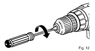
Insert allen wrench in chuck and tighten chuck jaws securely. Tap sharply with a mallet in a counterclockwise direction. This will loosen chuck on the spindle. It can now be unscrewed by hand. See Figure 13.
